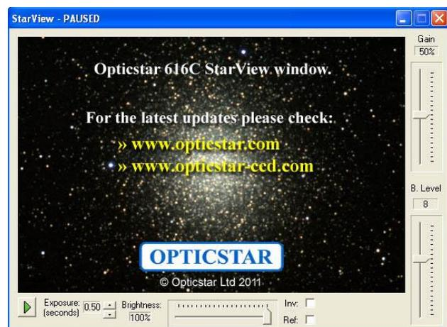
The **Offset** value controls the camera's **Black Level**. Typically, high data values contain more noise (bad data) than signal (useful data). The user can adjust this setting to modify at runtime the cut-off point between signal and noise. The most appropriate Offset value depends on many factors including the exposure time, gain value, the target, the binning mode, etc.
